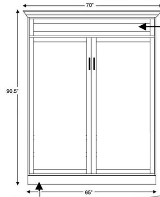
TO OPEN—WHEN YOU LIFT THIS PANEL FOOT YOU UNLATCH THE BED FROM THE CABINET TOP. ONCE PARTIALLY OPENED THE SAFE PISTON LIFT SYSTEM TAKES OVER AND THE BED SLOWLY LOWERS TO THE FLOOR
